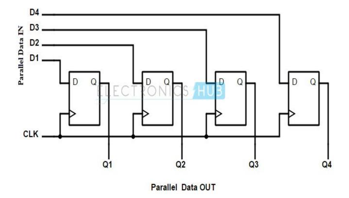
The above diagram shows the 4 stage parallel in parallel out register. Qa, Qb, Qc and Qd are the parallel outputs and Pa, Pb, Pc and Pd are the individual parallel inputs. There are no interconnections between any of the four flip flops. उपरोक्त आरेख parallel in
