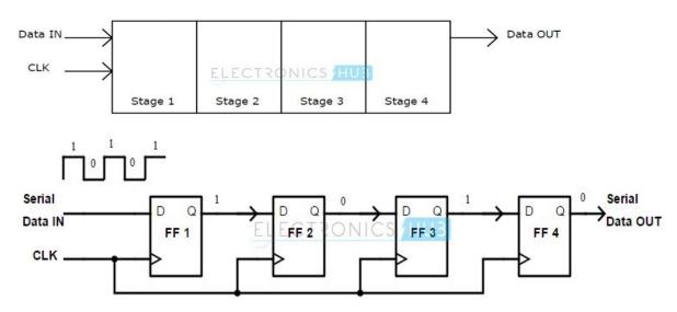
This one is the simplest register among the four types. the clock signal is connected to all the 4 flip flops. the serial data is connected to the left most or right most flip flop. The output of the first flip flop is connected to the input of the next flip flop and so on. The final output of the shift register is collected at the outmost flip flop.
