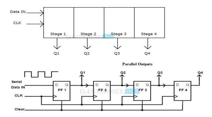
The clear (CLR) signal is connected with all the 4 flip flops to RESET the flip flop and the serial data is connected to the flip flop at either end (depending on shift left register or shift right register). The output of the first flip flop is connected to the input of the next flip flop and so on. All the flip flops are connected with a common clock.
